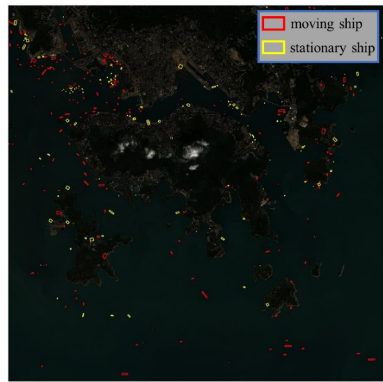
Figure 3. The ship monitoring results of Sentinel 2 image, which the red and yellow box indicates the position of the moving and stationary ship, respectively.
